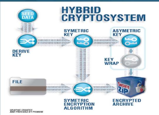
SecureZIP is implemented as a hybrid cryptosystem.
